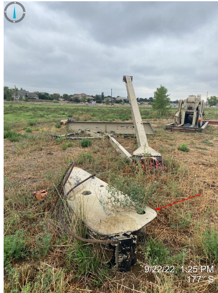
Photo 2. Close up photo of pump jack equipment. Alfalfa growing up through equipment indicates it has been stored and unused for a period of time.
