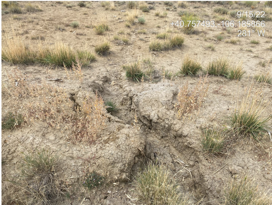
Photo 5. Photo taken from the northwest of the Location shows erosion occurring at the perimeter berm.
