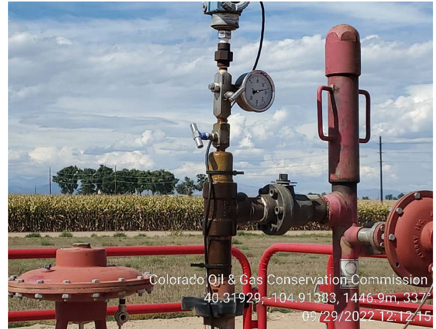
Lubricator outlet leak
