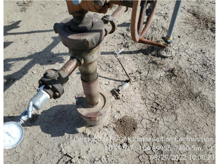
Walters 23-21DU master valve leak and stained soil
