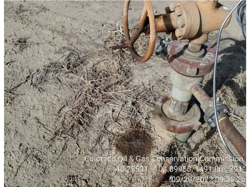
Ryland 20XD master valve leak and stained soil
