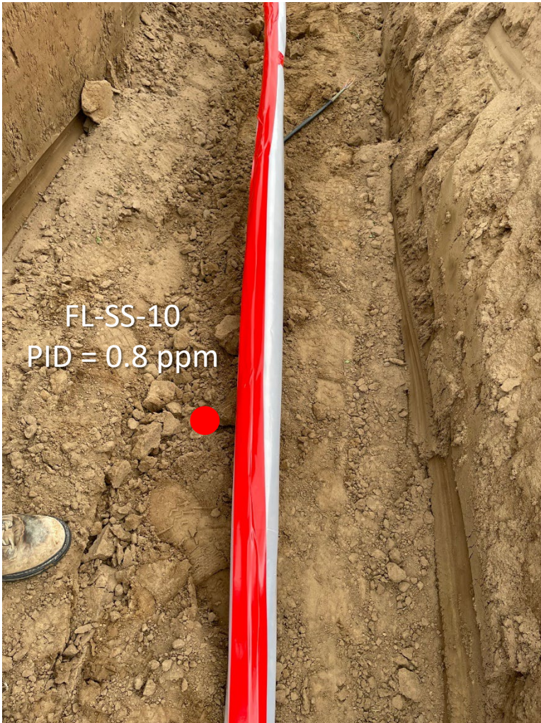
Looking northwest No petroleum hydrocarbon staining or odor observed
