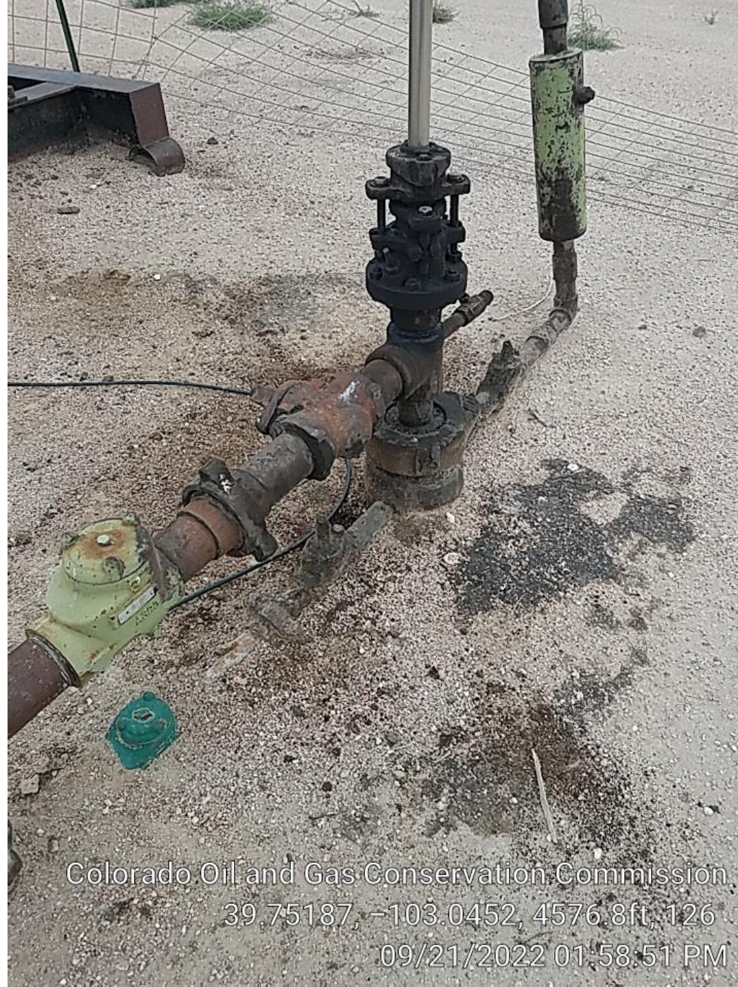
Stained soil at wellhead.
