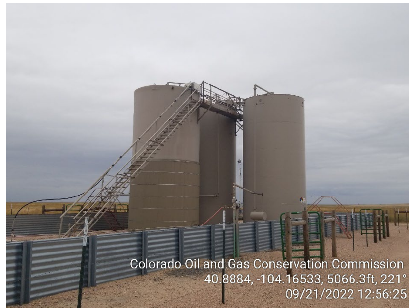
Photo 2 – Tank Battery
