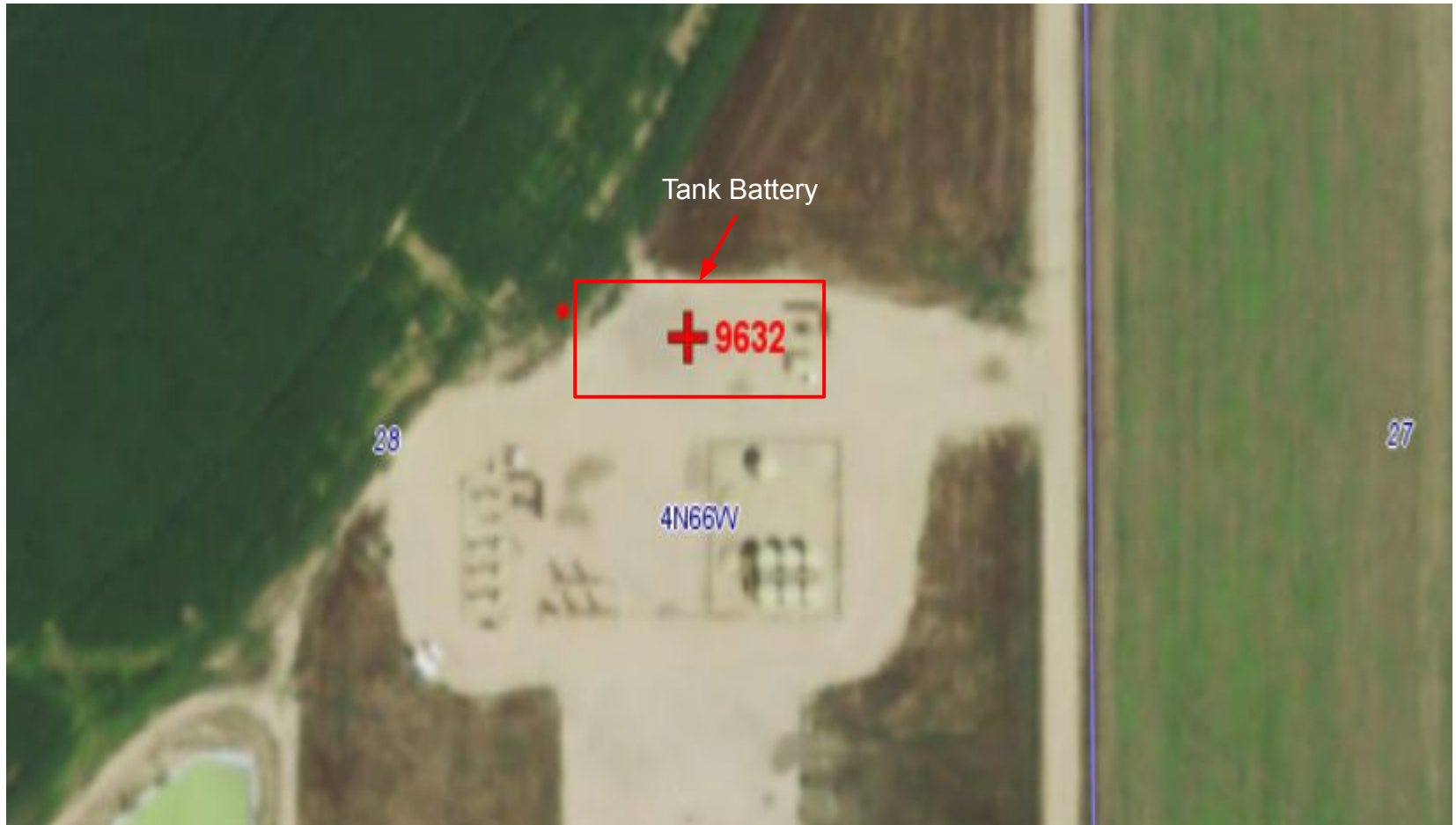
Photo 5. Open remediation at tank battery. Spill remediation under document #200439420. Monitoring wells were observed on site during the inspection. Tank Battery status will remain in-process until remediation has closed and location can be re-inspected.
