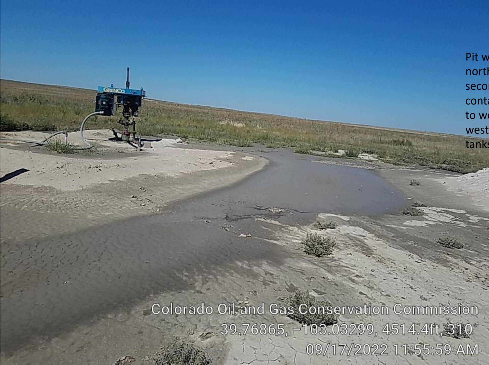
Pit water ran north over secondary containment to well and west or oil tanks.
