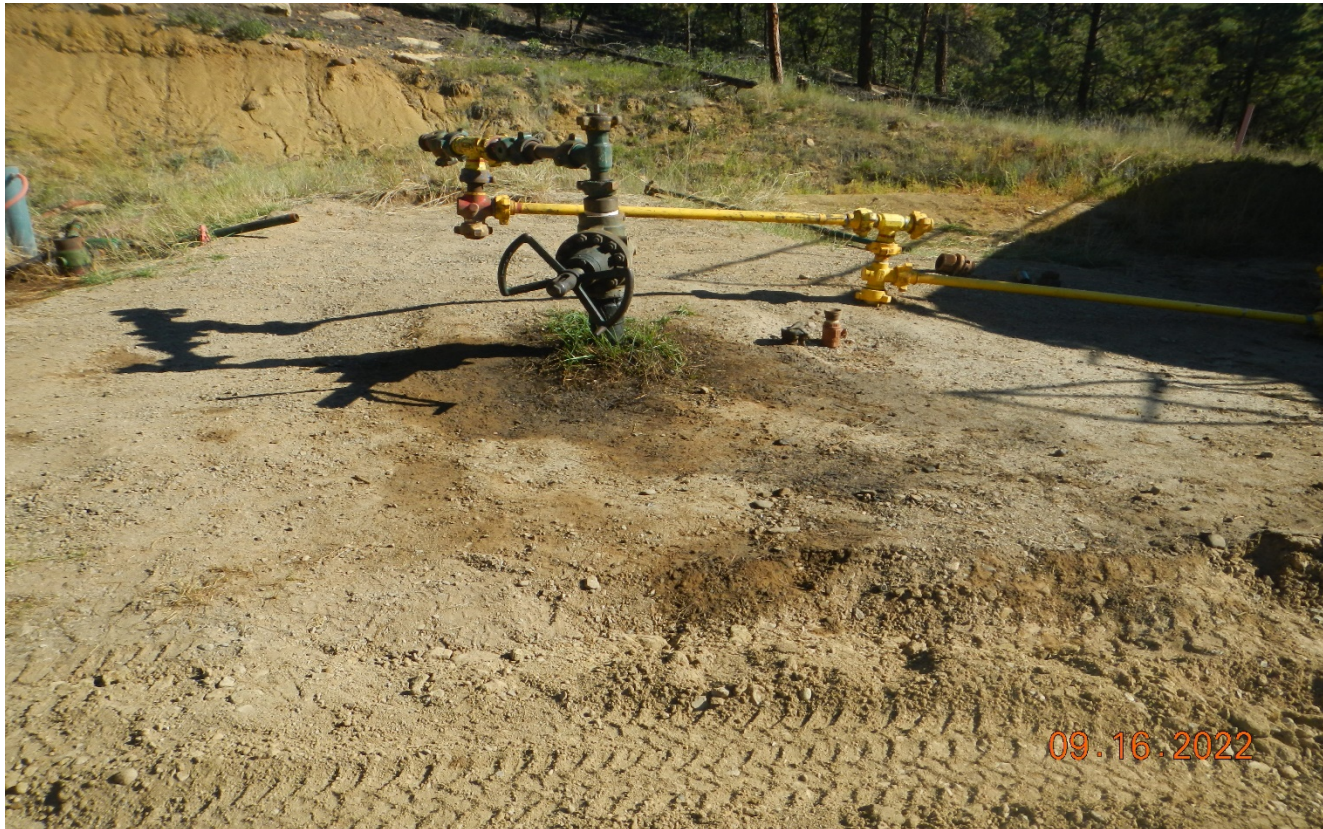
Photo 3. There are oil stained soils at the wellhead that must be cleaned up.
