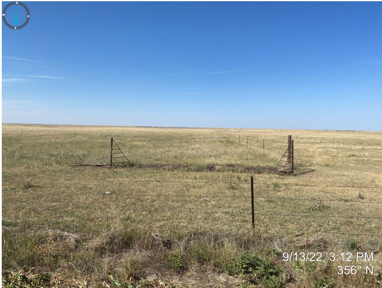
Photo 1. Photo taken from county road, facing north. Photo illustrates cattle guard remains at old access road entrance; fencing on perimeter of location remains. This material is now considered equipment/debris and needs to be removed.
