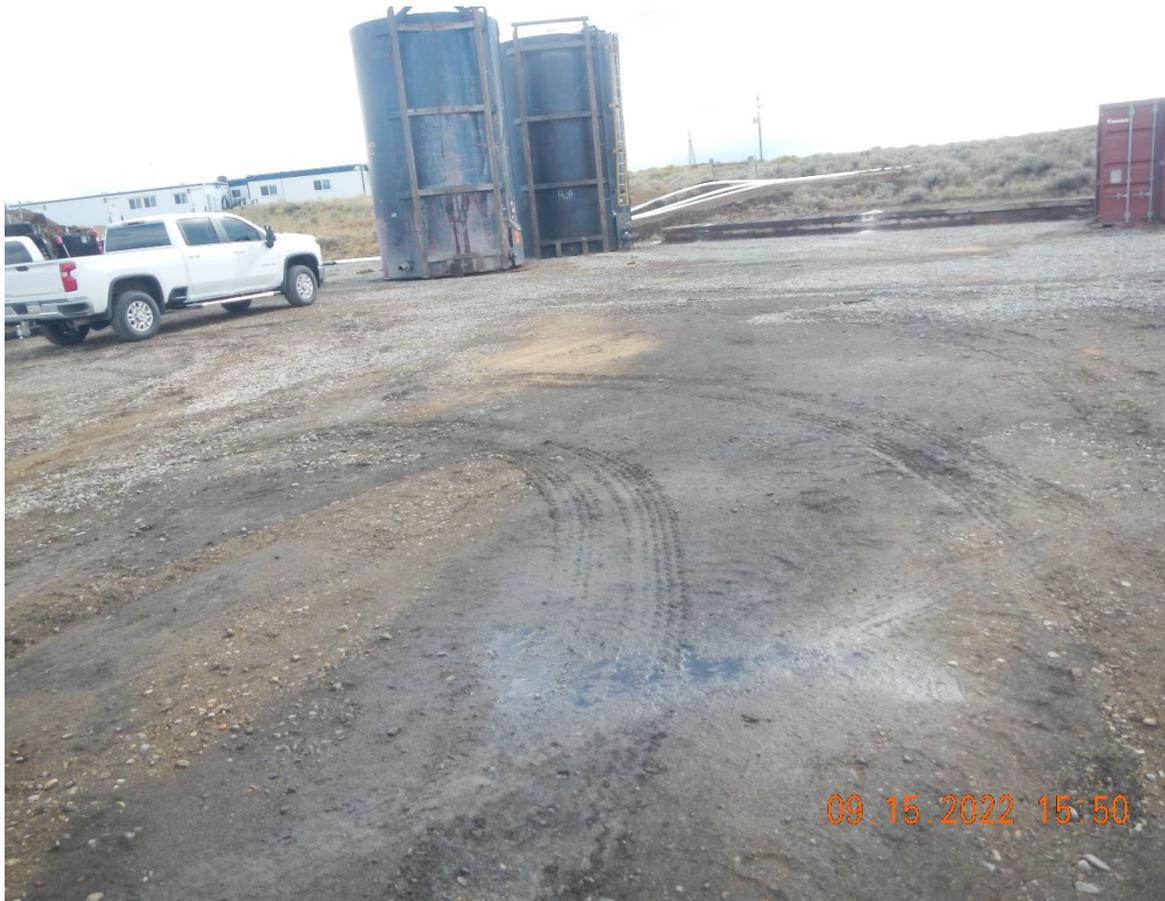
**Photo #2 black on the pad appears to be cuttings that have been driven into the pad.**
