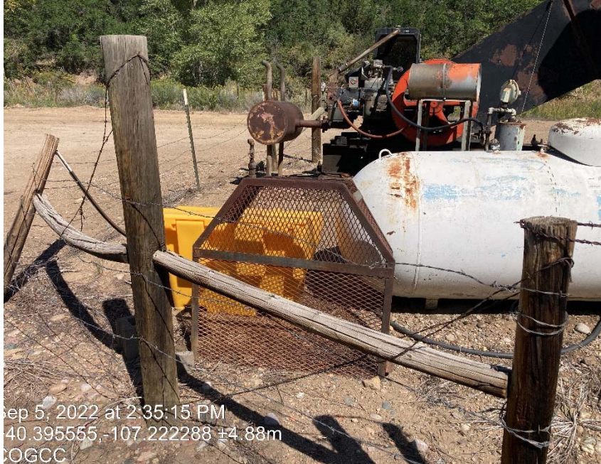
Propane tank lacking labeling/ Guard for pump jack
