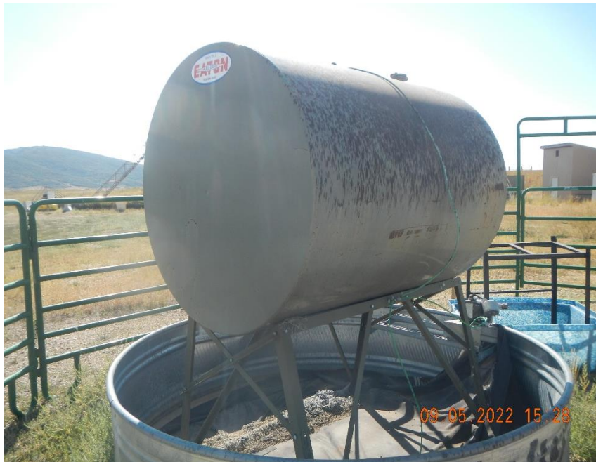
Methanol tank label is faded and missing information required for tanks over 10 bbls. Unused equipment including 2 tank stands, and 1 secondary containment tank were observed stored at the well area.
