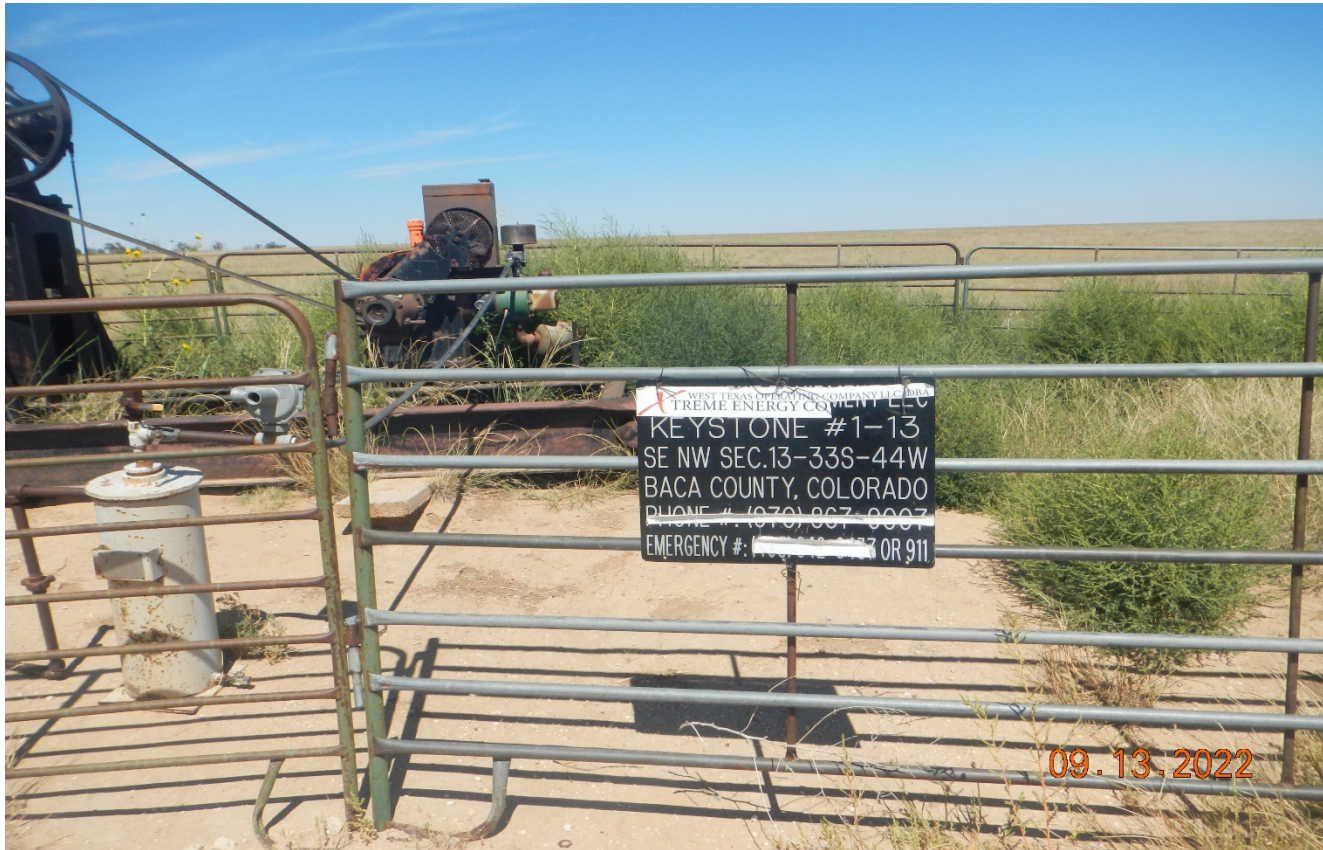
Photo 5. Well sign is posted by the pumpjack. The taped sign is peeled and faded and there is no emergency contact number.
