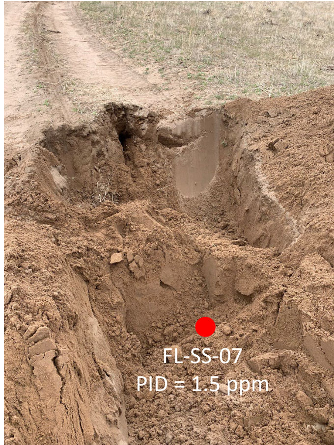
Looking southeast Bellhole/cut point – field screened No petroleum hydrocarbon staining or odor observed
