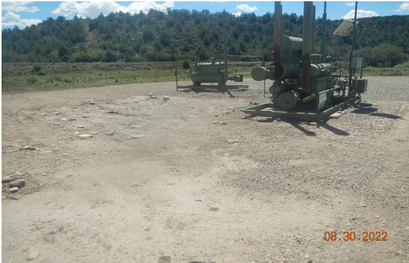
Photo 2. Facing southeast toward Bondad 33-9 equipment. The open top tank has been removed from this site. The remaining equipment needs to have improved secondary containment installed.
