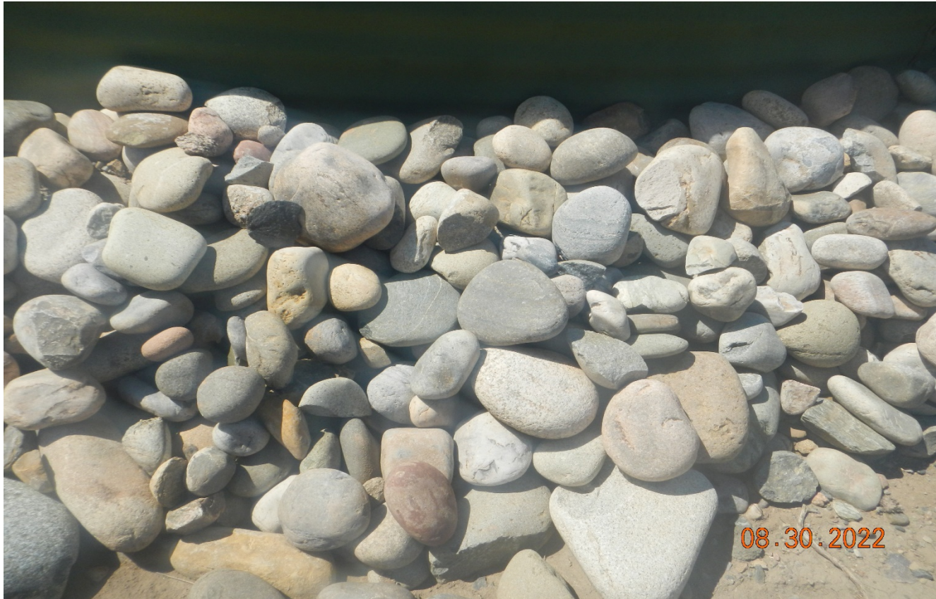
Photo 3. The round rock is pervious and will not prevent flood water from entering underneath the steel containment. Round rock will also be easily displaced as they do not lock in place as well as angular rock. Another solution needs to be implemented.
