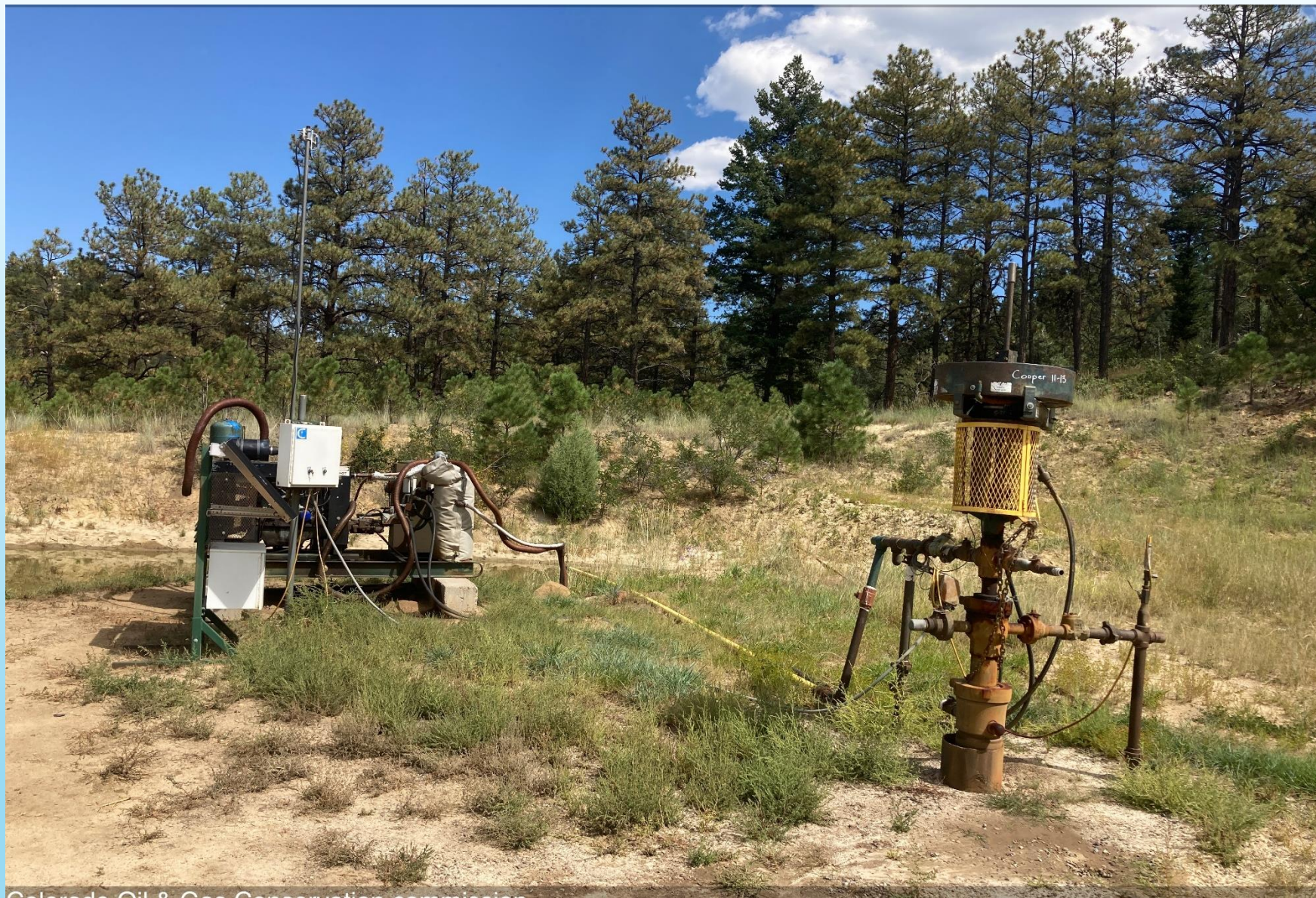
PHOTO 3: ORIGINAL WELLHEAD AND EQUIPMENT
