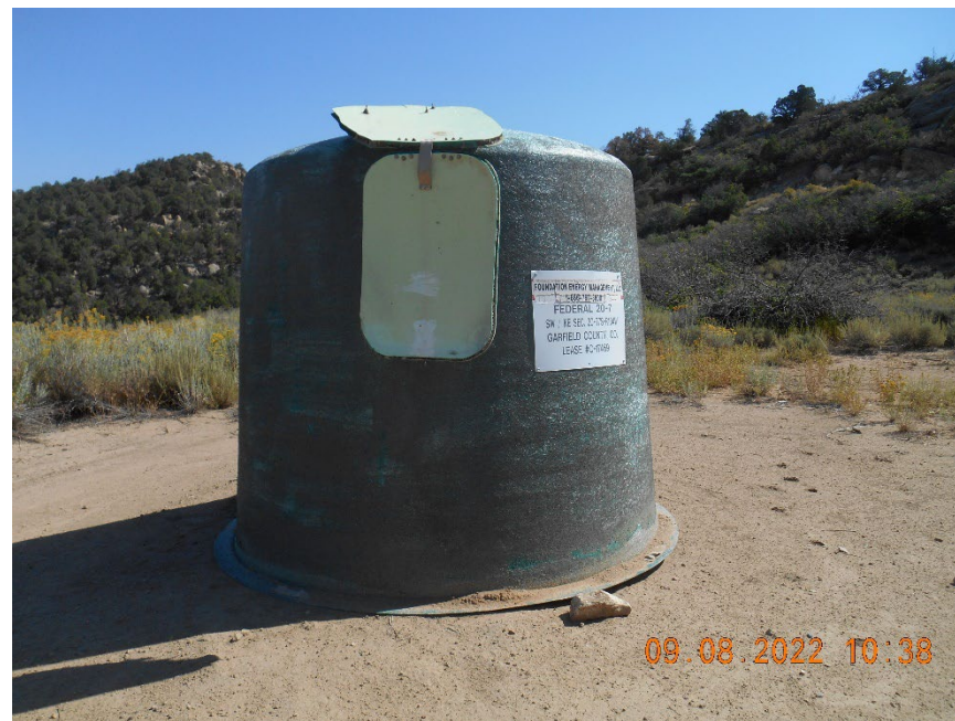
Wellhead inside fiberglass housing
