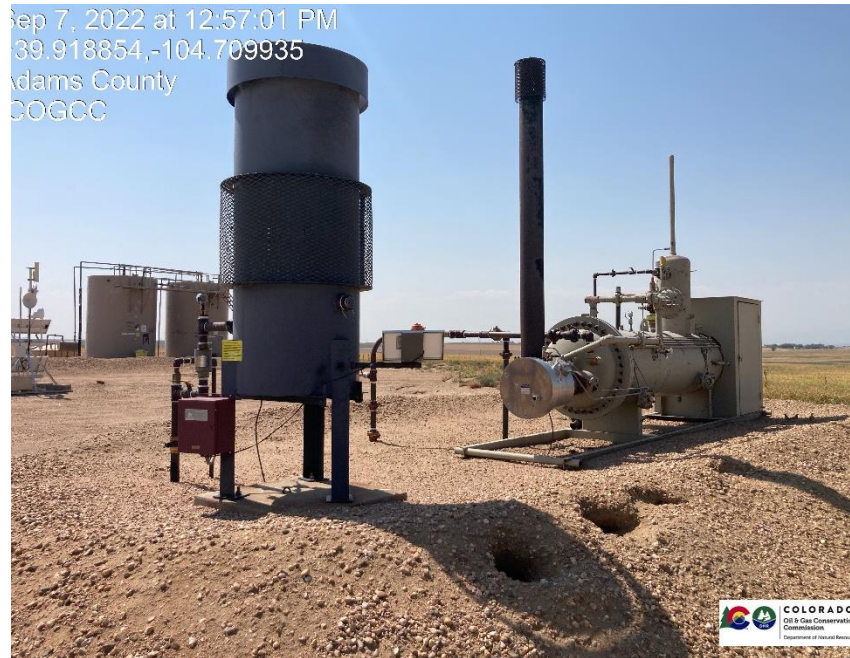
Pic 3 ECD, Separator
