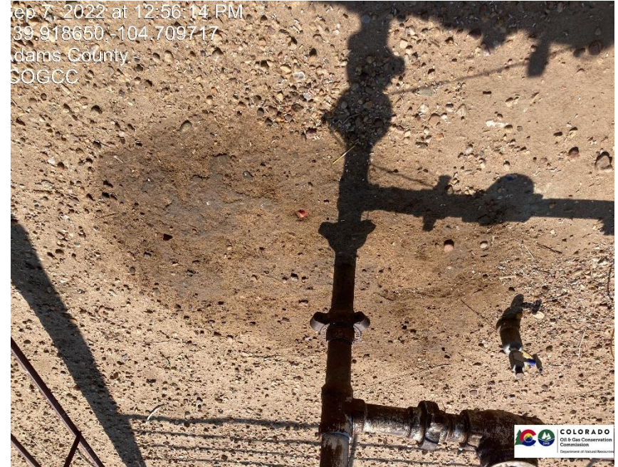
Pic 2 Stained soil by wellhead flowline
