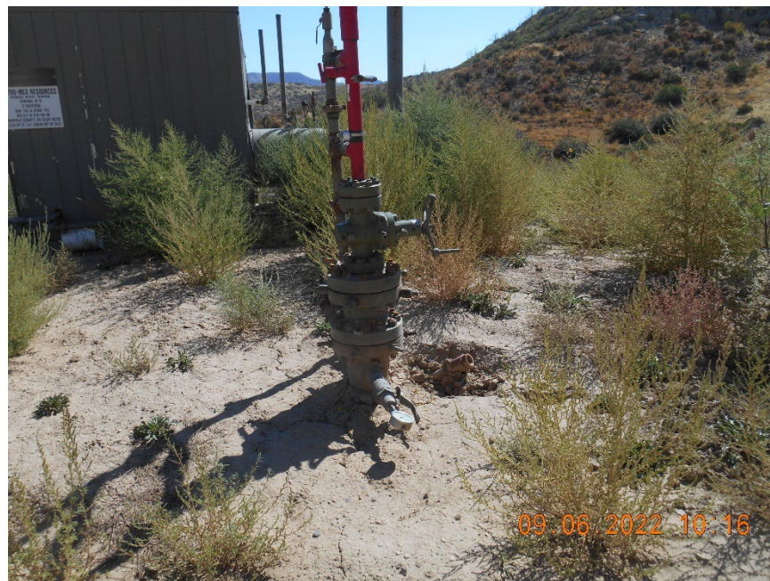
Wellhead bradenhead valve exposed
