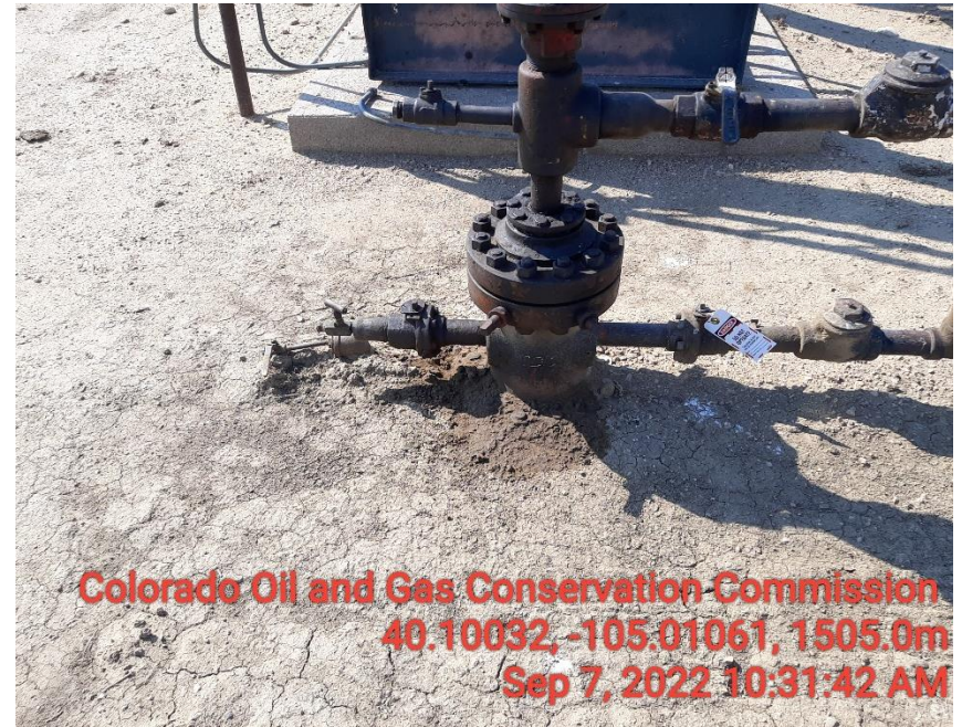
Photo 4 stained soil around well head
