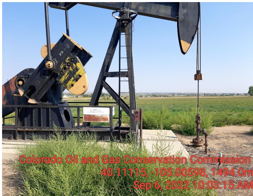
Photo 3 Well head sign unreadable and weeds around equipment
