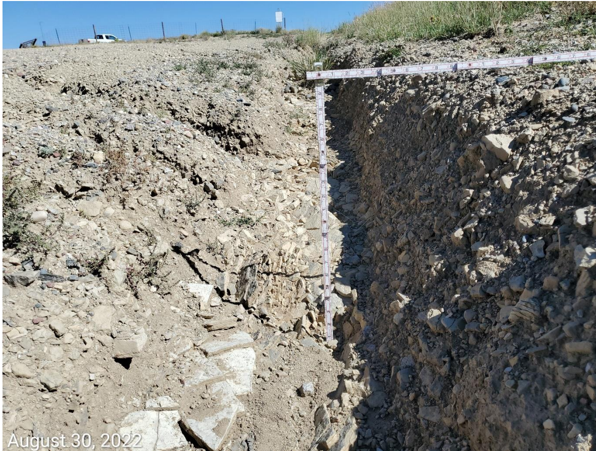
Photo 7: Photo taken from the access road. Photo shows gully erosion at access road is ~2 feet deep.
