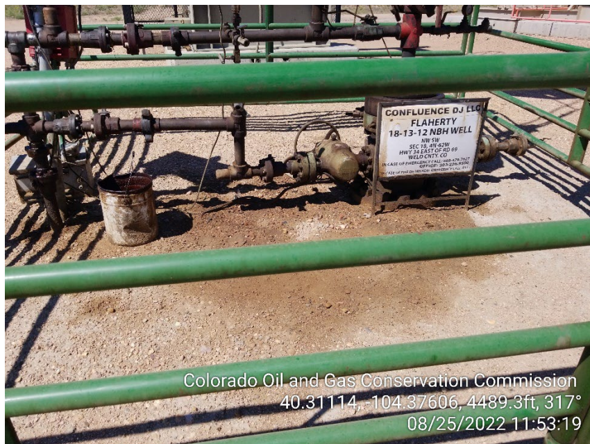
Photo 1 – 18-13-12 Wellhead – Stained Soil
