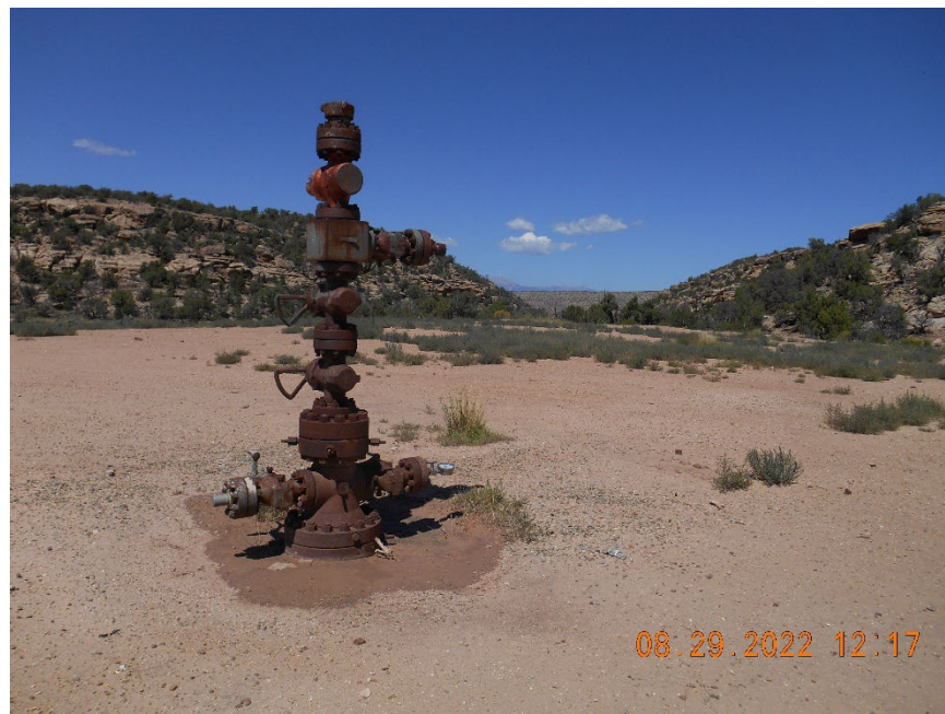
Wellhead . Temporarily abandoned
