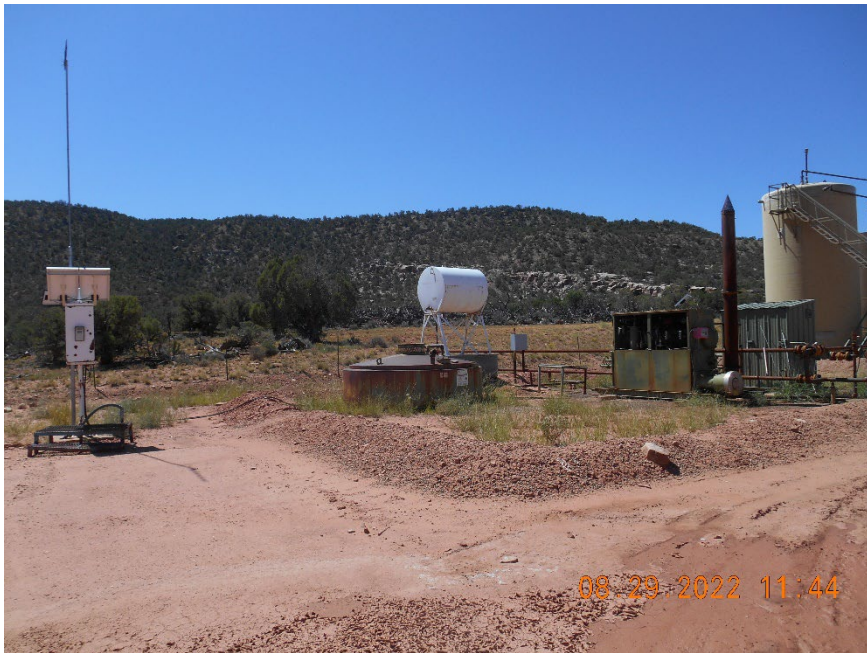
Separator, Meter housing and Blowdown tank
