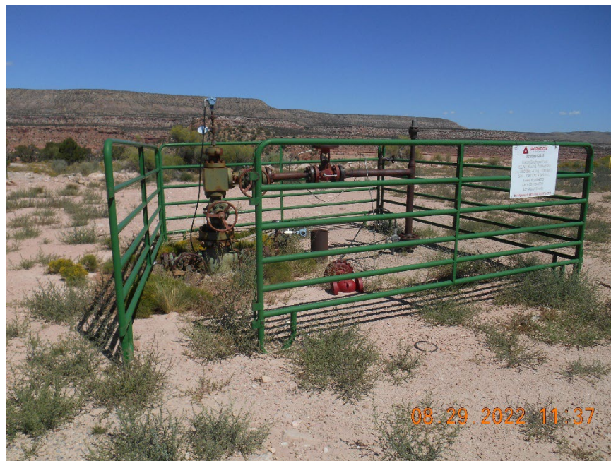
Wellhead with fence and sign
