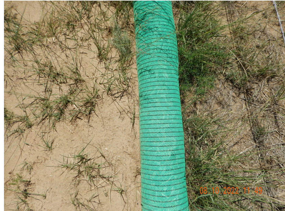
Photo 4. Photo taken along a portion of the western location. Photo illustrates how the filtrex wattle properly worked to keep sediment from leaving location.
