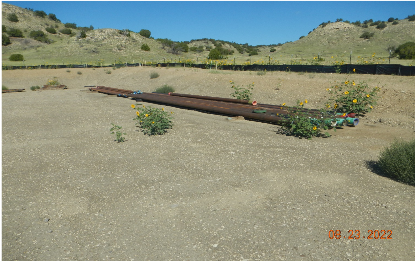
Photo 12. The drilling pipe needs to be remove per rule 606.
