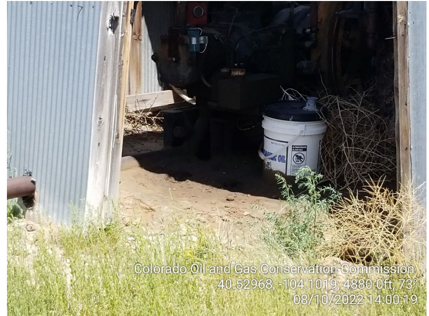
Photo 4 – Stained Soil at Gas Engine
