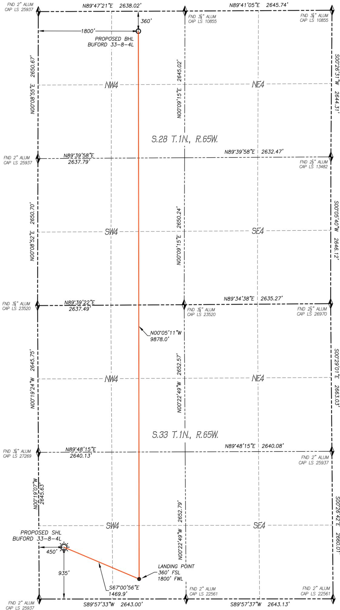
IN ACCORDANCE WITH A REQUEST FROM CONFLUENCE RESOURCES, DALEY LAND SURVEYING, INC. HAS DETERMINED THE SURFACE LOCATION OF THE BUFORD 33-8-4L WELL TO BE 935' FSL, 450' FWL, AS MEASURED AT NINETY (90) DEGREES FROM THE SECTION LINES OF SECTION 33, TOWNSHIP 1 NORTH, RANGE 65 WEST AND THE BOTTOM HOLE LOCATION TO BE 360' FNL, 1800' FWL, AS MEASURED AT NINETY (90) DEGREES FROM THE SECTION LINES OF SECTION 28, TOWNSHIP 1 NORTH, RANGE 65 WEST, OF THE 6TH PRINCIPAL MERIDIAN, WELD COUNTY, COLORADO.
