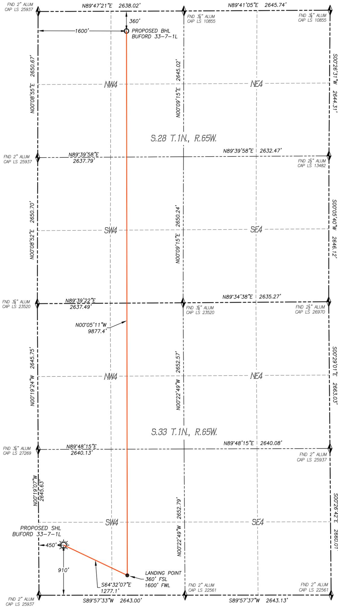
IN ACCORDANCE WITH A REQUEST FROM CONFLUENCE RESOURCES, DALEY LAND SURVEYING, INC. HAS DETERMINED THE SURFACE LOCATION OF THE BUFORD 33-7-1L WELL TO BE 910' FSL, 450' FWL, AS MEASURED AT NINETY (90) DEGREES FROM THE SECTION LINES OF SECTION 33, TOWNSHIP 1 NORTH, RANGE 65 WEST AND THE BOTTOM HOLE LOCATION TO BE 360' FSL, 1600' FWL, AS MEASURED AT NINETY (90) DEGREES FROM THE SECTION LINES OF SECTION 28, TOWNSHIP 1 NORTH, RANGE 65 WEST, OF THE 6TH PRINCIPAL MERIDIAN, WELD COUNTY, COLORADO.
