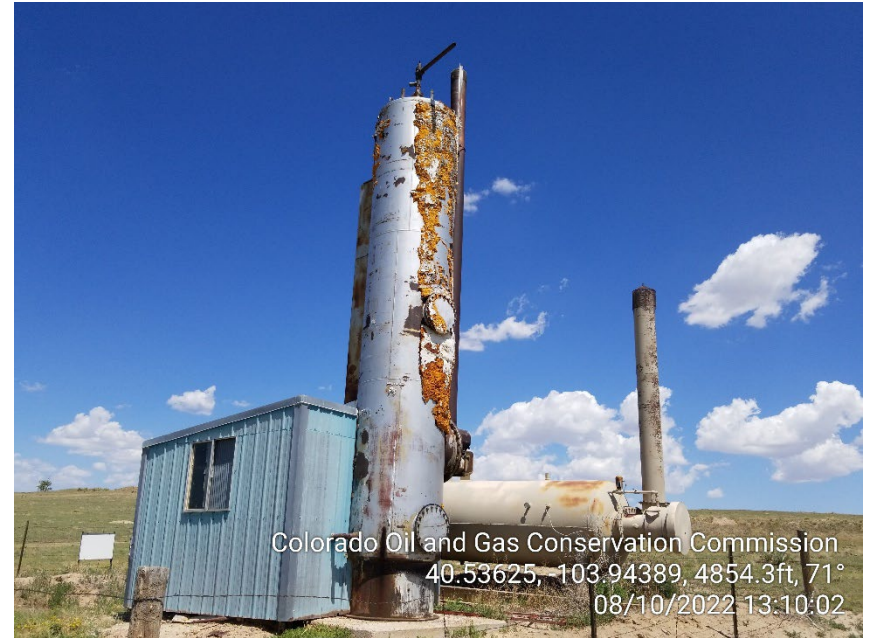
Photo 6 – Separator and Heater
