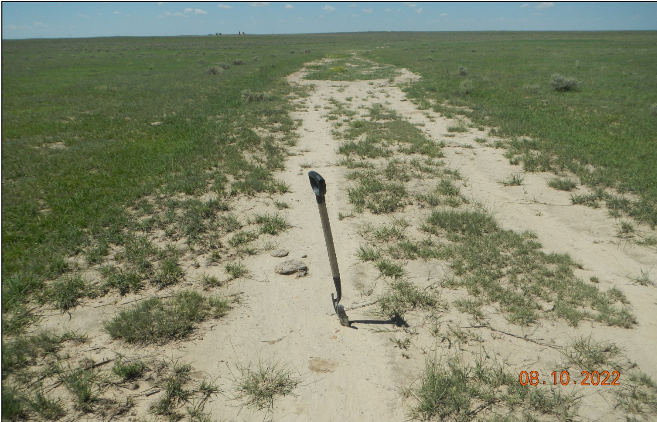
Photo 2. Facing west toward the access road which needs to be decompacted and reclaimed. Shovel could not penetrate soil surface as shown.
