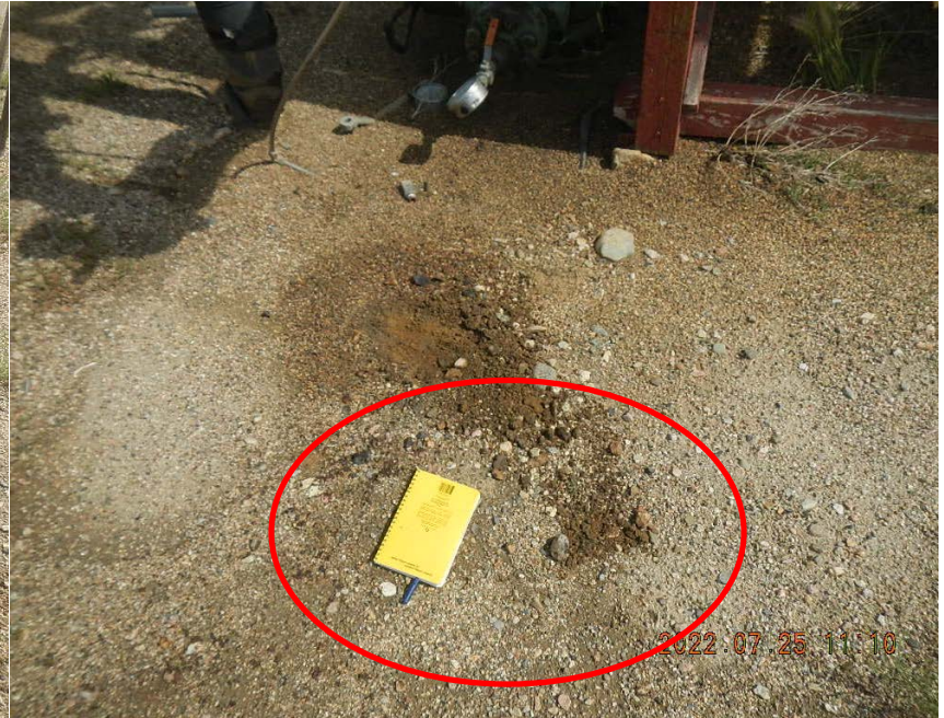
Staining from May 2021 gas leak/vent and condensate around wellhead. Apparent newer material imported over previously impacted area.
