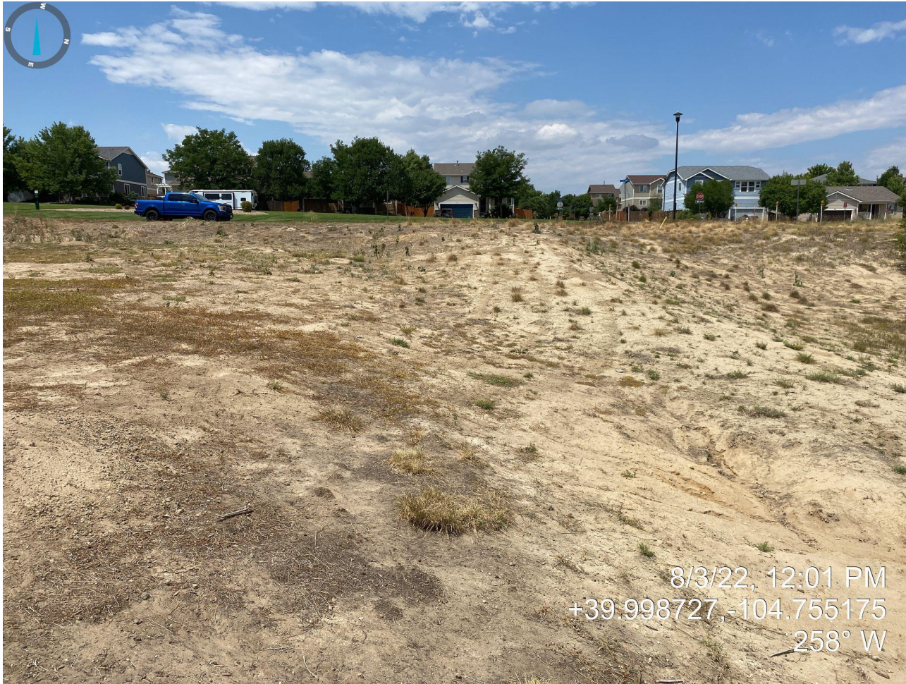
Photo 2. Location photo taken from northern portion, facing west. Photo illustrates lack of uniform vegetation cover resulting in bare soil.
