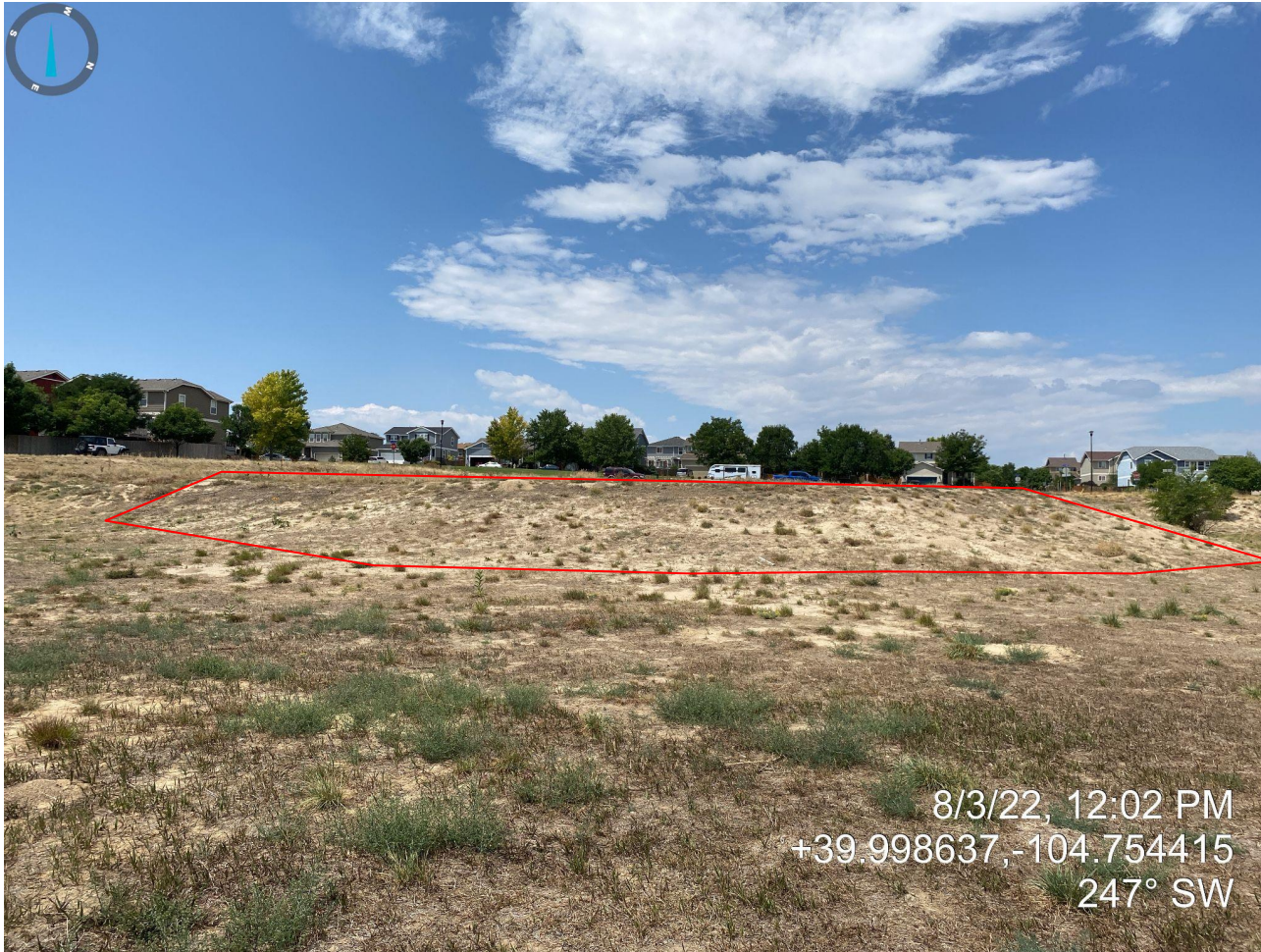
Photo 3. Photo taken east of location, facing southwest. Photo illustrates that location (highlighted in red) and access road have not been reclaimed (e.g. not regraded or recontoured).
