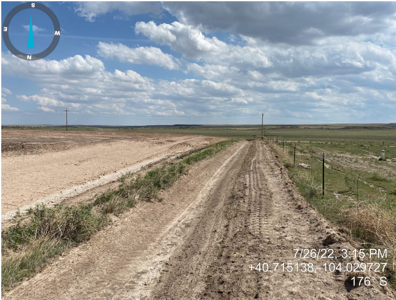
Photo 7. Location photo taken from western portion, facing south. Photo illustrates ditch and berm BMP installed during construction phase.
