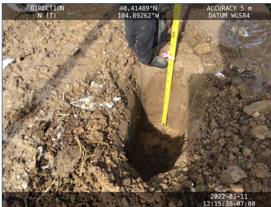
Photograph 9. Topsoil depth pit (TSCS20) with topsoil determined to be at 9 inches. Change in color from medium brown to a lighter gray-brown. Soil texture became more compact.
