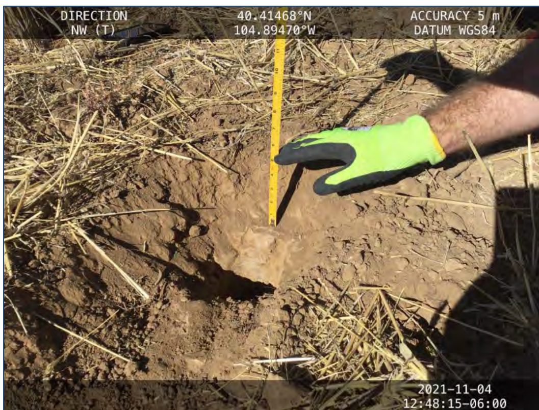
Photograph 2. Topsoil depth pit (TSCS 3) with topsoil determined to be at 5 inches. Change in color from light-medium brown to a lighter gray-brown. Soil texture became more compact with “shelving.”
