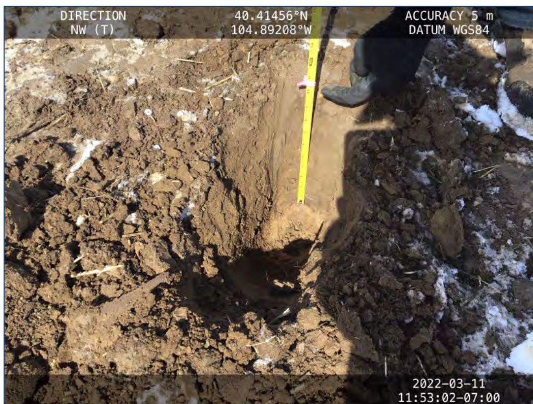
Photograph 10. Topsoil depth pit (TSCS21) with topsoil determined to be at 10 inches. Change in color from medium brown to a lighter gray-brown. Soil texture became more compact.
