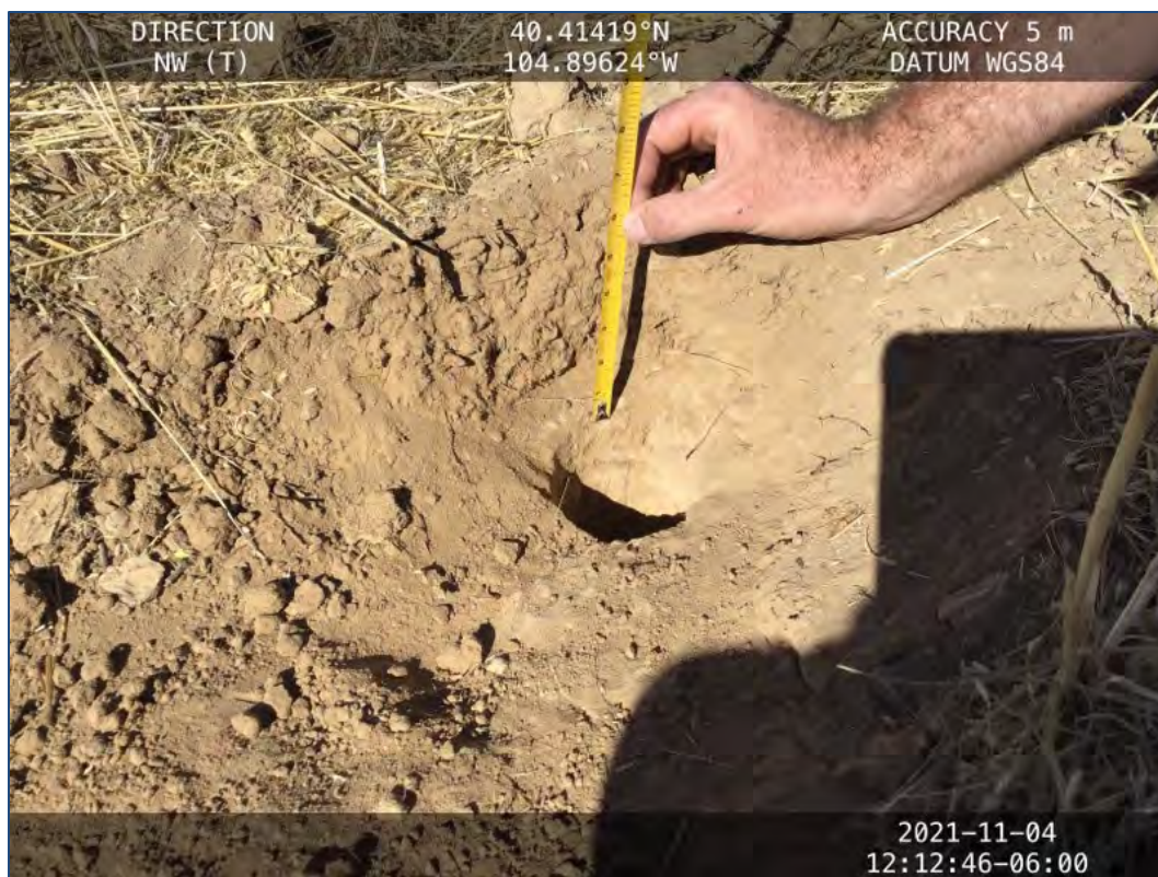
Photograph 3. Topsoil depth pit (TSCS 4) with topsoil determined to be at 6 inches. Change in color from light-medium brown to a lighter gray-brown. Soil texture became more compact with “shelving.”
