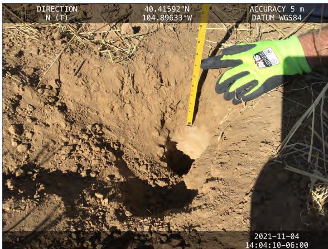
Photograph 1. Topsoil depth pit (TSCS 1) with topsoil determined to be at 7 inches. Change in color from light-medium brown to a lighter gray-brown. Soil texture became more compact with some “shelving.”
