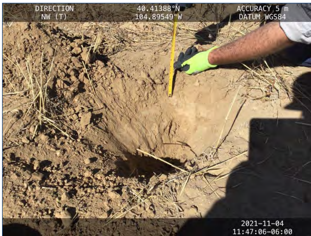
Photograph 4. Topsoil depth pit (TSCS 5) with topsoil determined to be at 5 inches. Change in color from light brown to a lighter gray-brown. Soil texture became more compact.
