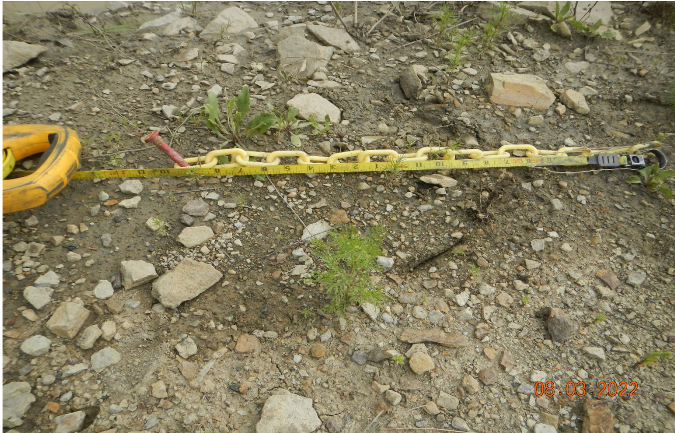
Photo 4. The freeboard marker is not is not 2ft. In length and does not show the vertical depth where it is installed. (Lays on the slope of the ground)
