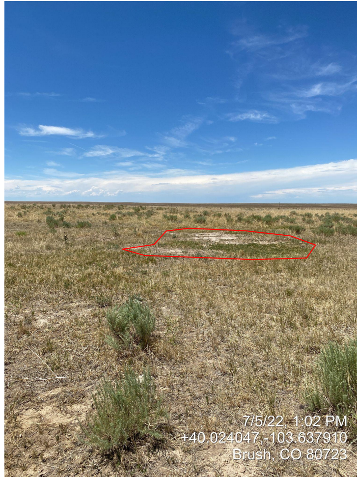
Photo 3. Location photo taken from eastern portion, facing west. Subsidence (highlighted in red) observed around well location and non-uniform vegetation cover resulting in bare soil.
