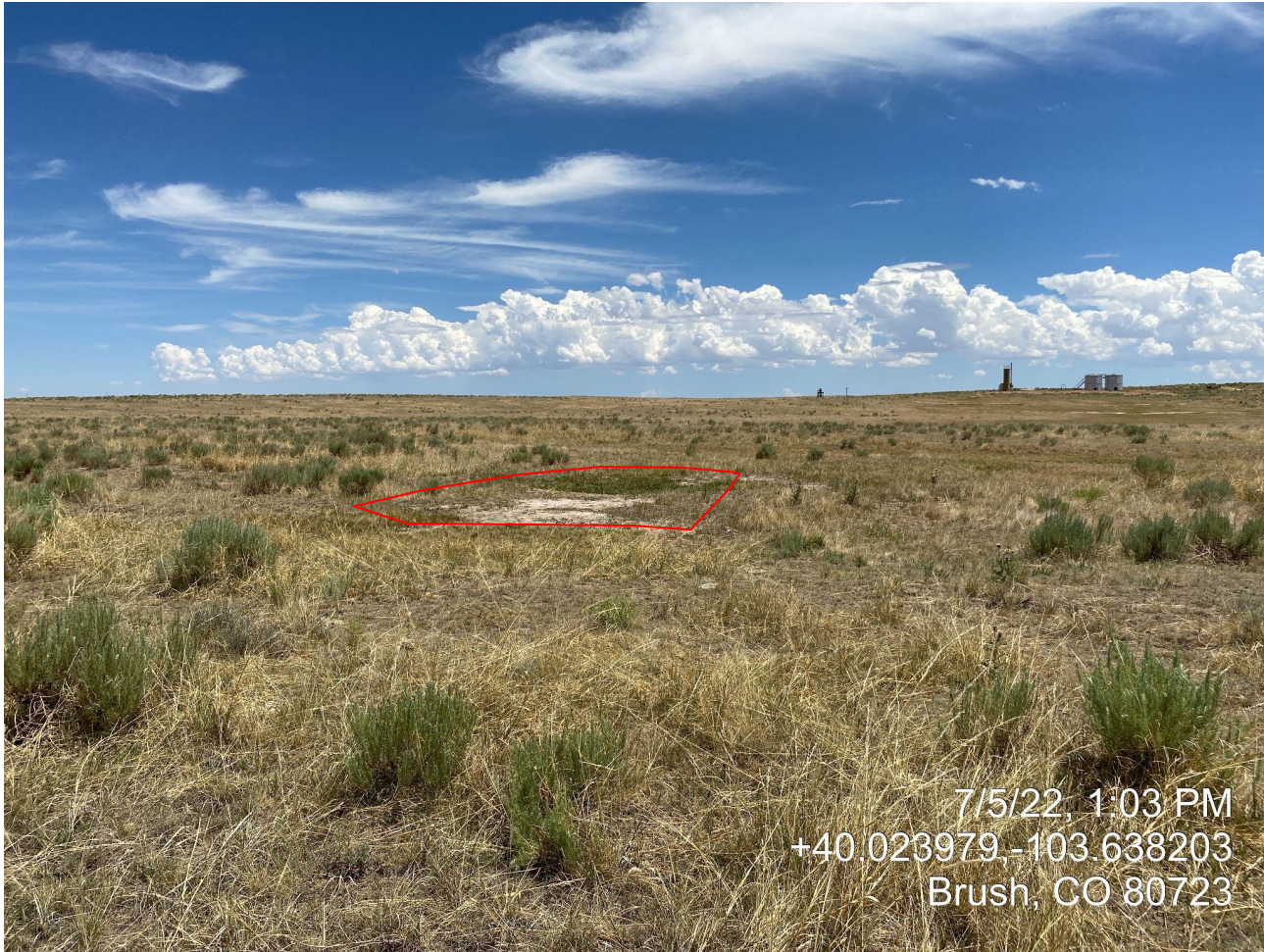
Photo 5. Location photo taken from western portion, facing east. Subsidence (highlighted in red) observed around well location and non-uniform vegetation cover resulting in bare soil.
