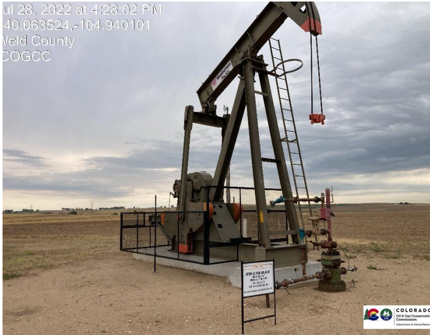
Pic 1 wellhead / pump jack / plunger lift
