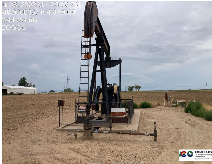
Pic 1 pump jack / wellhead
