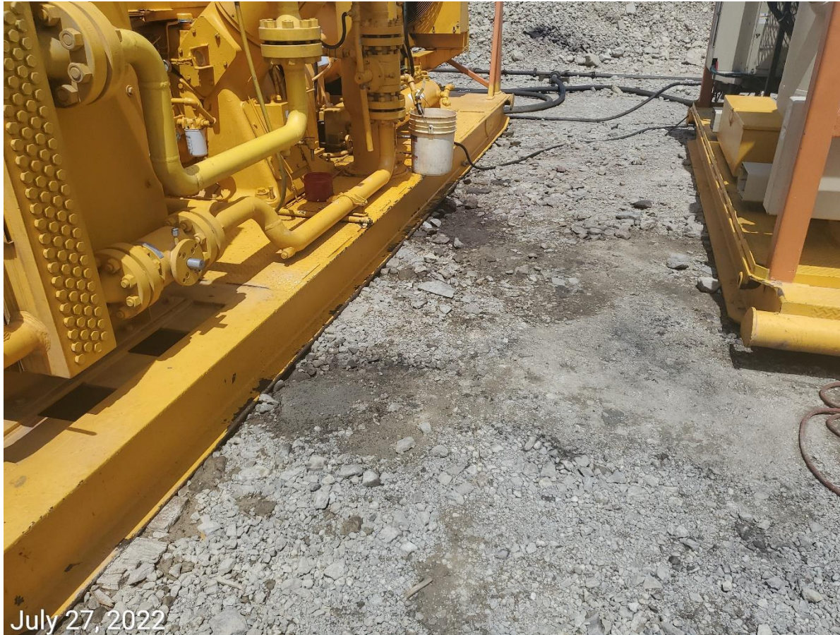
Photo 2: Photo shows impacted soils due to spills from equipment.
