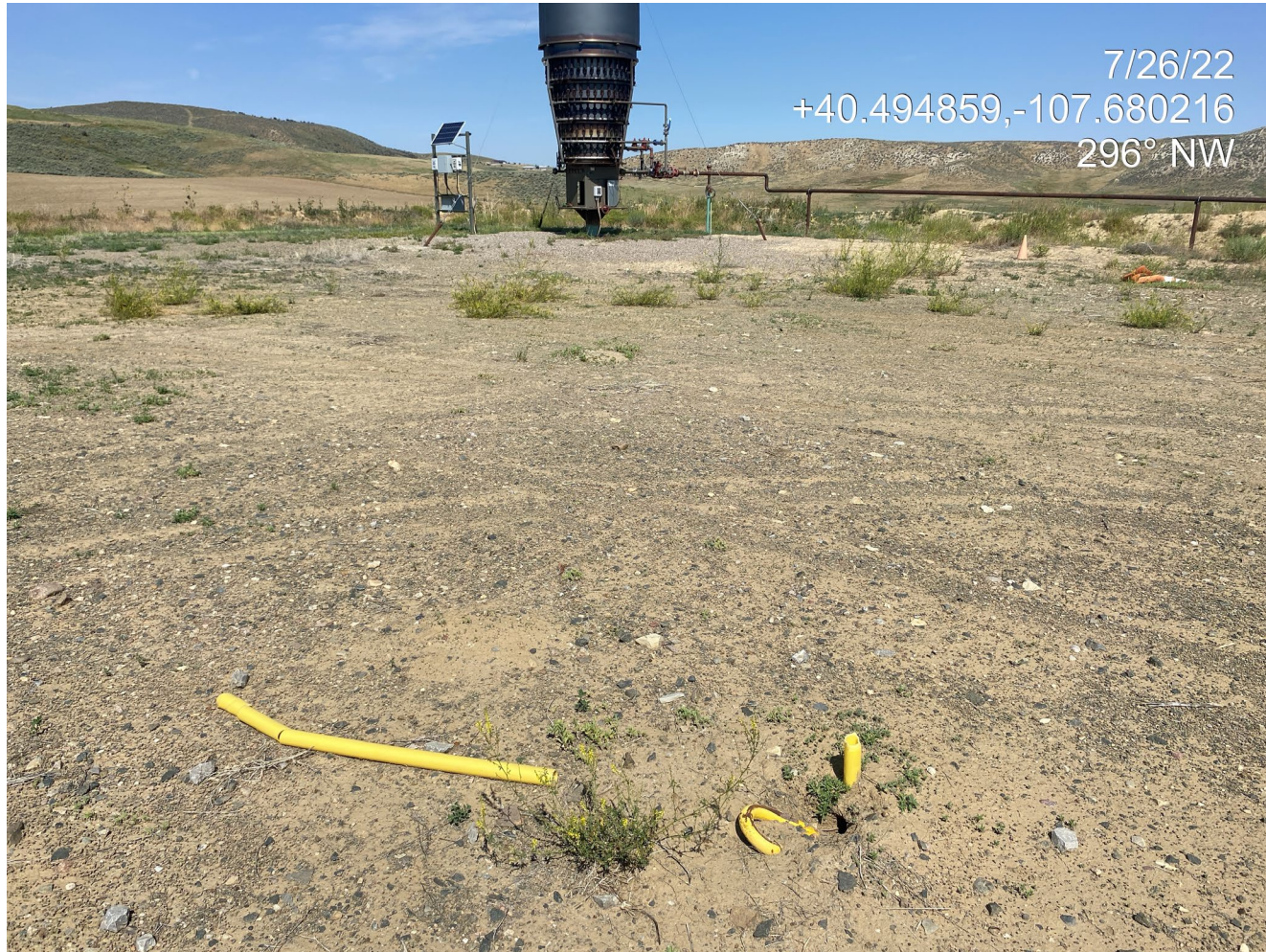
Photo 8. Photo taken from the northwest of the Location shows an anchor marker in disrepair. Four anchor markers on Location were observed in disrepair.
