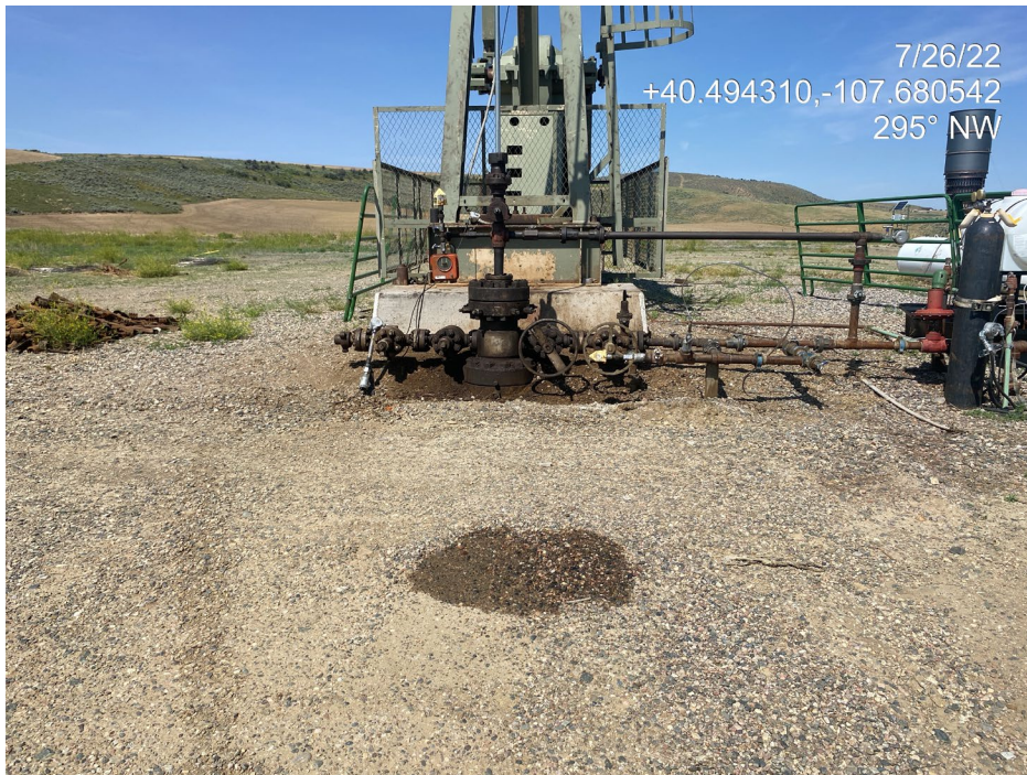
Photo 4. Photo taken from the wellhead shows stained soils.
