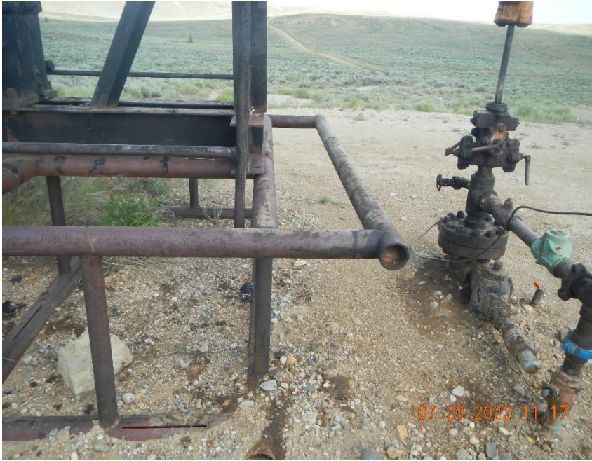
Oil stained ground at pumpjack and well.
