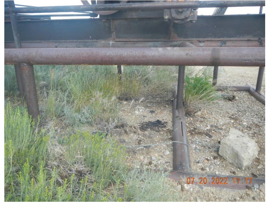
Oil stained ground at well. Weeds growing around pump jack.
