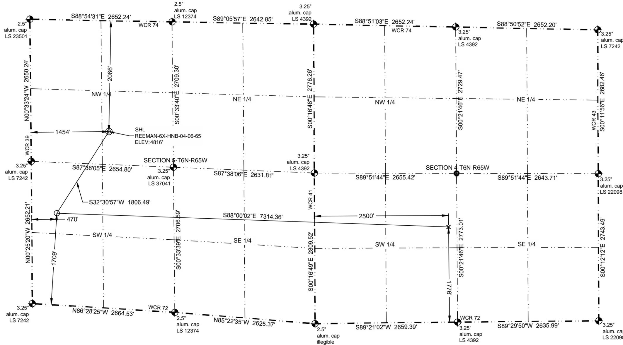
In accordance with a request from Kit Tincer of Nickel Road Operating LLC, Sterling Land Surveyors, LLC has determined the location of the **REEMAN-6X-HNB-04-06-65** well site to be SHL: 2066' FNL and 1454' FWL, (LPL: 1709' FSL and 470' FWL), (BHL: 1776' FSL and 2500' FWL), as measured at ninety (90) degrees from the section lines of Sections 4 and 5, Township 6 North, Range 65 West of the 6th Principal Meridian, Weld County, Colorado.
