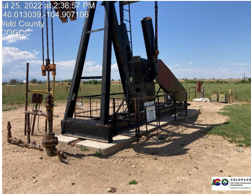
Pic 1 Pump jack / wellhead
