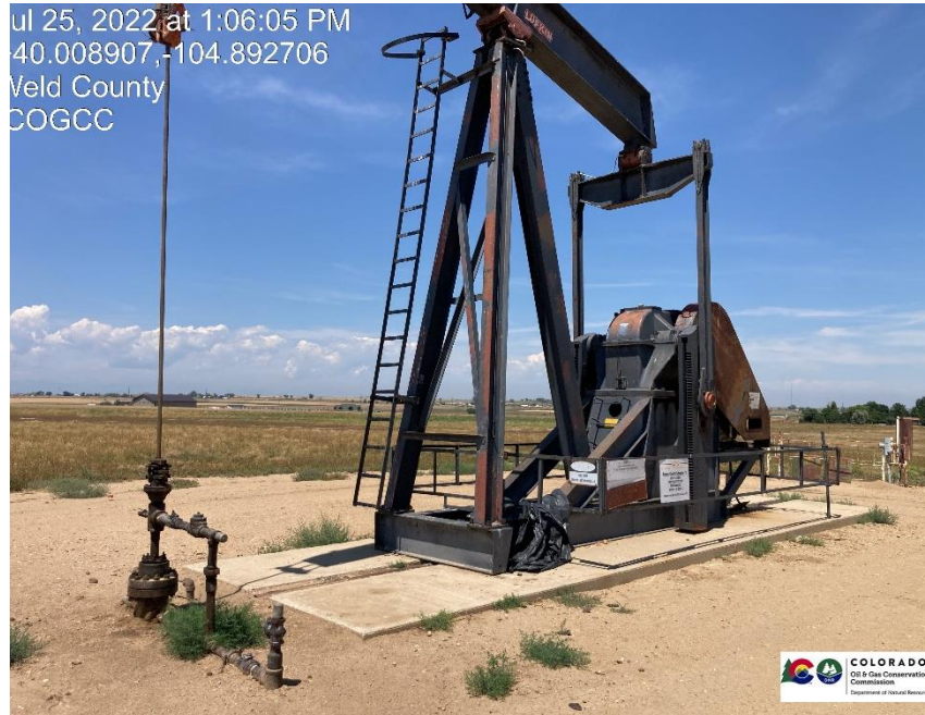
Pic 1 wellhead / pump jack
